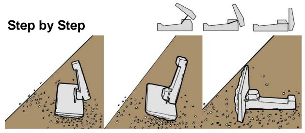
**Retaining Module Assembly**
